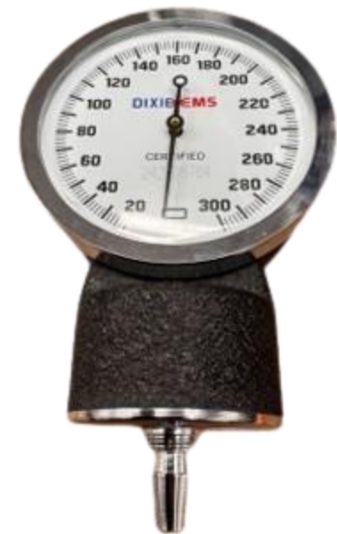
Figure 7. Pressure gauge used to determine appropriate brace tightness.
